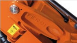
Articulated joints with drop forged parts
